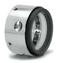
These Seals can be easily assemble or dismantled through circlip provided & cab be change to Balance version of its type merely by changing the carbon face only & an be provided with single, double or tandem arrangement worth external seal support systems & devices.
