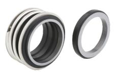
seal can be use regardless of direction of rotation since the driving torque is not transmitted through the coil spring, The required driving torque is enhanced through the unique rubber bellow which fits on the shaft. There are no bonded Joints and all the face materials are interchangeable without having to modify any dimensions.
